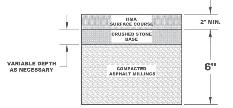
NOTE: COMPACTED STONE BASE ONLY REQUIRED IN EVENT DEPTH OF ASPHALT MILLINGS DOES NOT MEET MINIMUM PAVING CROSS-SECTION REQUIREMENTS
