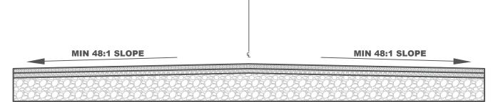
NOTE: IN THE EVENT THAT EXISTING ROADWAY DOES NOT PERMIT TYPICAL ROADWAY CROSS-SECTION, THE CONTRACTOR IS RESPONSIBLE FOR PROVIDING ROADWAY CROSS SECTION THAT PERMITS POSITIVE DRAINAGE WITH APPROVAL OF THE ENGINEER
